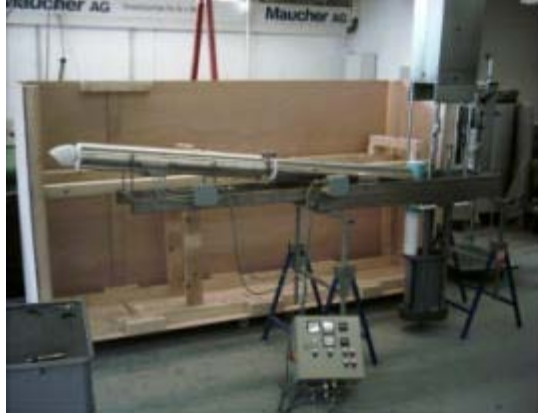
picture 9 pumping equipment for liquid metal pumping and metering
