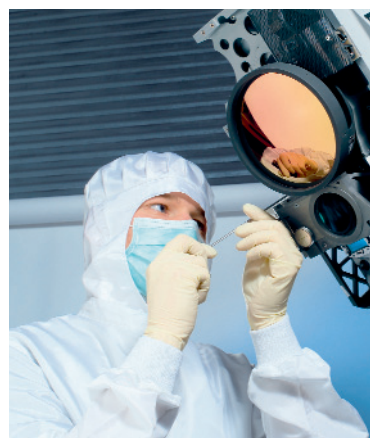
Fig. 1 Housing structure (l.) and final assembly of an avionic reconnaissance telescope camera (r.)
