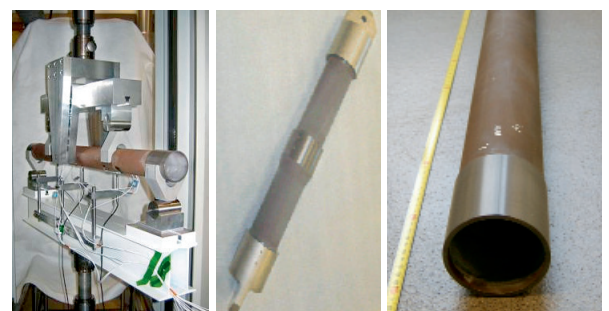
Fig. 5 Testing set up for silicon nitride beams and connected beams for satellite truss structure
