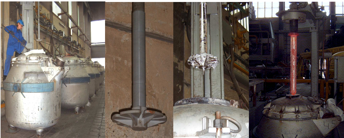
Fig. 2_Example for foundries: degassing impeller and immersion heater sheath for a transport Aluminium tank
